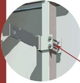
Window mold is designed to hang from ties.
