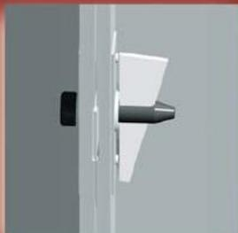
Our round, tapered pins have a milled wedge slot. The shank is designed to eliminate pin sag and improve ease of stripping. Pins are made from steel and are heat-treated for long life.
