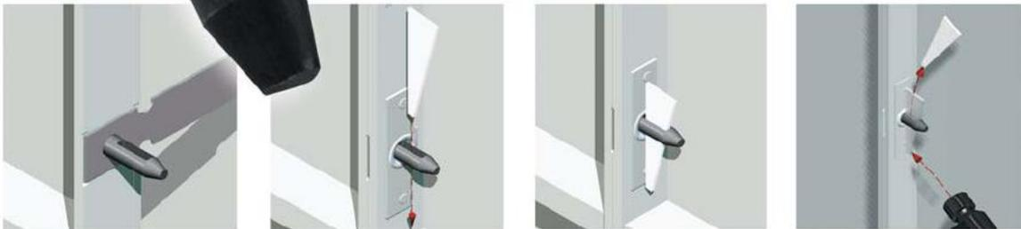
Typical connection with pin and straight wedge.
