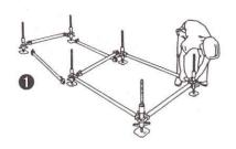
1. Select the highest ground level of desired work area. Screw nut near bottom of shank and set in base collars in desired geometry. Lay out ledgers and transoms between base collars. Assemble wedges lightly into collars without driving home the wedges.
